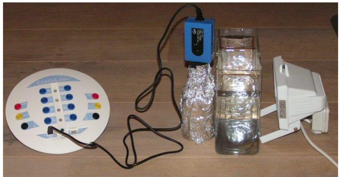
For the second ten minutes of the measurement (10 to 20 min), the aluminum foil is removed and the bottle is placed in ambient light (circa 700 Lux). The CO<sub>2</sub> gas concentration still increases but more slowly, with a rate of 44 ppm/min. More carbon dioxide is produced in respiration than there is used by photosynthesis.
