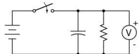
Figure 2. Electrical circuit for discharging a capacitor
