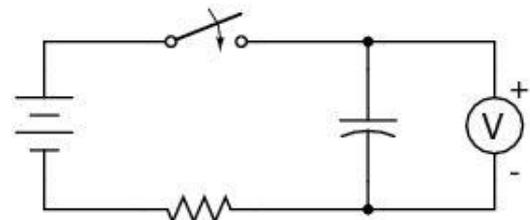
Figure 1. Electrical circuit for charging a capacitor
