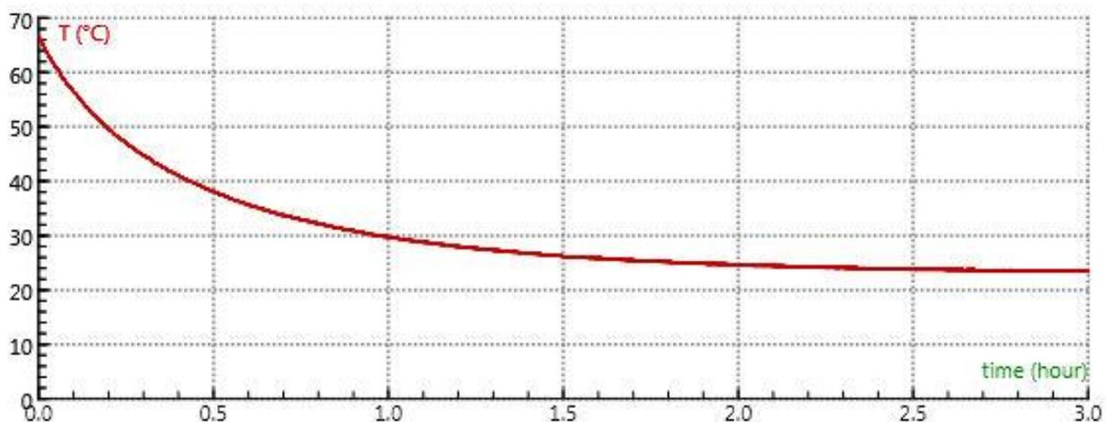
Temperature measurement during cooling down a cup of coffee.
