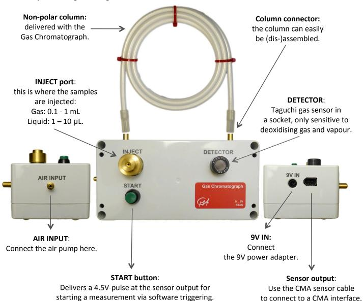
The GC BT45i can be directly connected to analog BT inputs of CMA interfaces. The sensor cable BT - IEEE1394 needed to connect the sensor to an interface is not supplied with the sensor and has to be purchased separately (Order Code BTsc 1).
