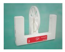
wheel measured in the groove is 0.20 m. On the edge of the groove the circumference is 0.21 m. Thus, the movement of a cord from the revolving pulley depends to some extent on the cord thickness. Calibration can be done by measuring the circumference with the used cord and dividing the length by 10, the number of spokes (the step size). Each time a new gap in the pulley is reached it corresponds to a displacement of this distance since the start of the
