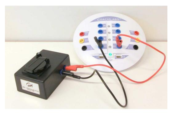
**Figure 2.** Connecting the switch module to the CoachLab II<sup>+</sup> interface.
