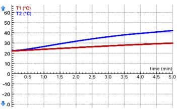
The sensor in the black test tube (blue graph) warms up faster than the sensor in the white test tube (red graph).
