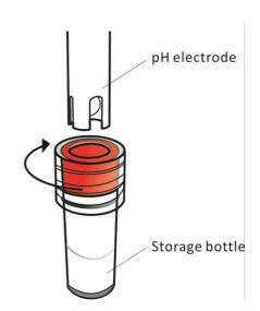
The pH electrode can be damaged beyond repair by improper use such as keeping the electrode in distilled water storage, usage over its temperature range and long-time exposure to strong acids/bases.
