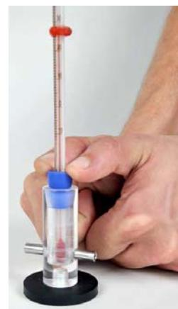
c) Fix the thermometer with the red silicone triangle to achieve a perpendicular positioning of the thermometer
