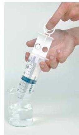
Step 8: Position the beaker under the open hose-connection of the heat exchanger. At the open hose-connection of the pump fill the circulation-flow-circuit with the help of the syringe. Smoothly press the syringe until the water streams out of the open hose-connection of the heat exchanger without bubbles.
