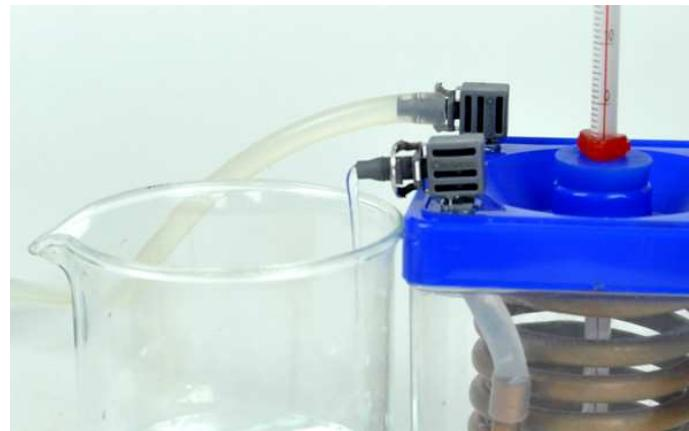
Step 9: Pull off the hose from the syringe and stick the open end onto the heat exchanger.
