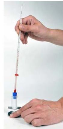
b) Adjust the height; the expansion vessel of the thermometer should not touch the ground.
