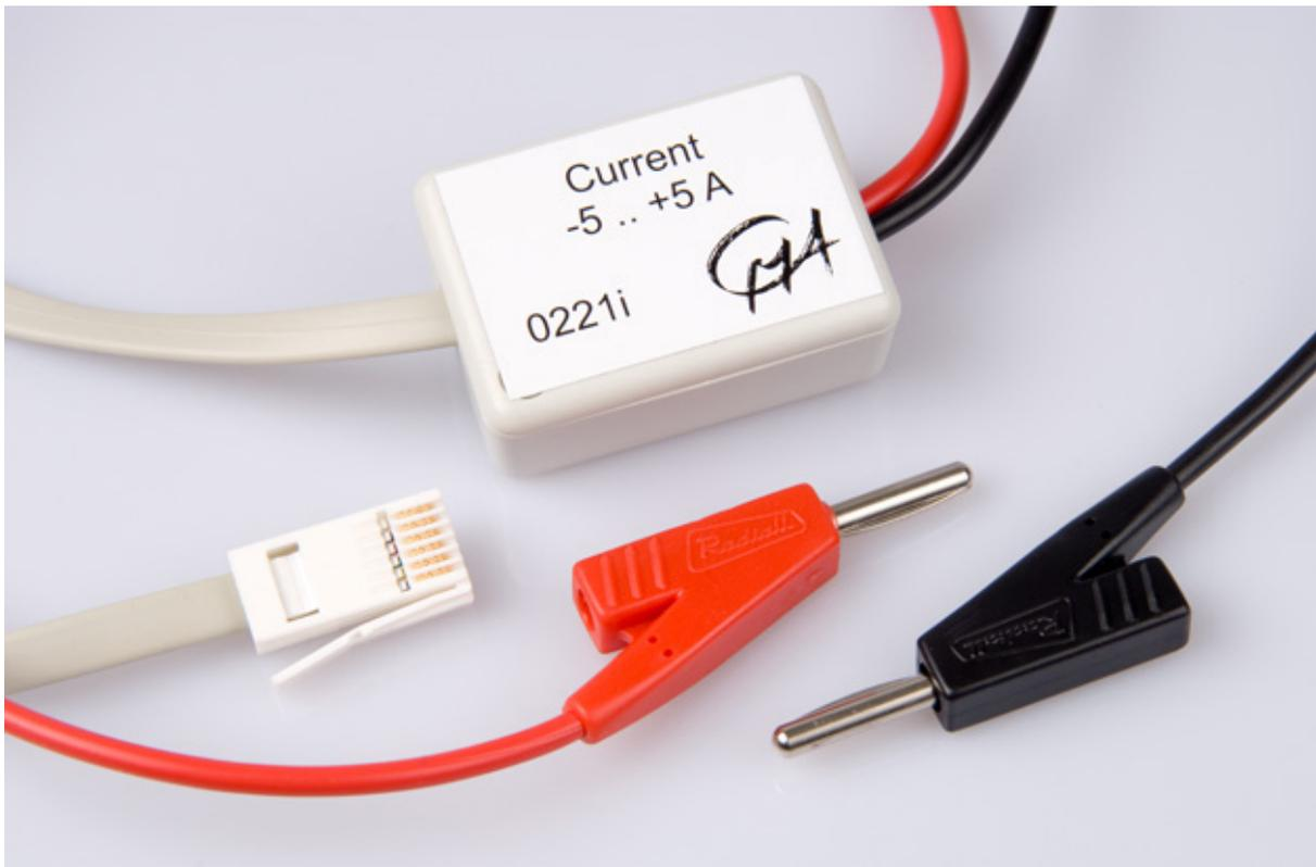
**Figure 1.** The Current sensor - 5 .. +5 A
